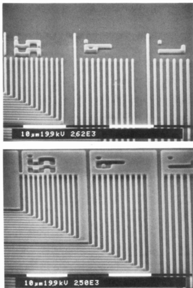
Figure 10. Scanning electron micrographs of images generated in a modified PBOCST/ \text{Ph}_3\text{SAsF}_6 formulation exposed on a 0.35 NA, 1X, UltraStep X-248E step-and-repeat projection system built by Ultratech. The dose was approximately 8 \text{ mJ}/\text{cm}^2 .
